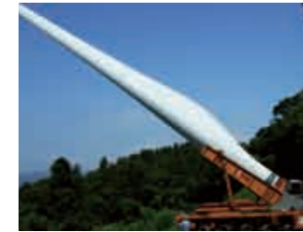
Blade erection equipment
