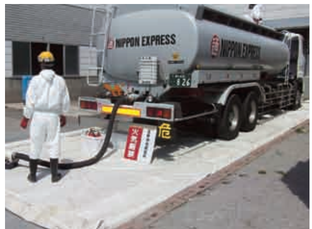
PCB delivery vehicle (tank lorry)
