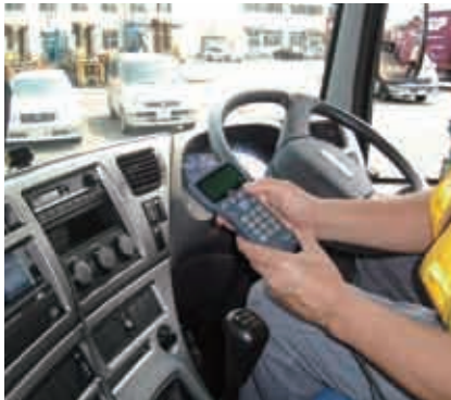
Installation of Digital Operation Recorders
